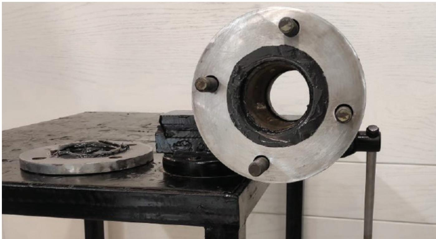
As an alternative method to welding processes, **HEGGEL Fix 831** is a repair/restoration putty which greatly decreases the risk of negative chemical or mechanical changes (mostly caused by heat affected zones (HAZ)) to the base materials, offering strong bonding and a clean result.
