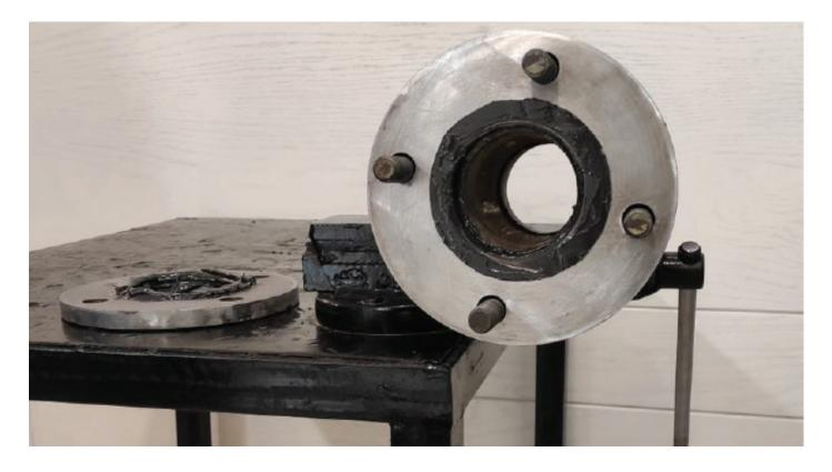
As an alternative method to welding processes, **HEGGEL Fix 831** is a repair/restoration putty which greatly decreases the risk of negative chemical or mechanical changes (mostly caused by heat affected zones (HAZ)) to the base materials, offering strong bonding and a clean result.
